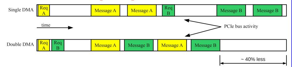
Doubling the number of transaction request on PCIe bus allows an efficiency gain in multiple data transactions (40% less time measured). will be presented at ReConFigurable Computing Conference 2013
