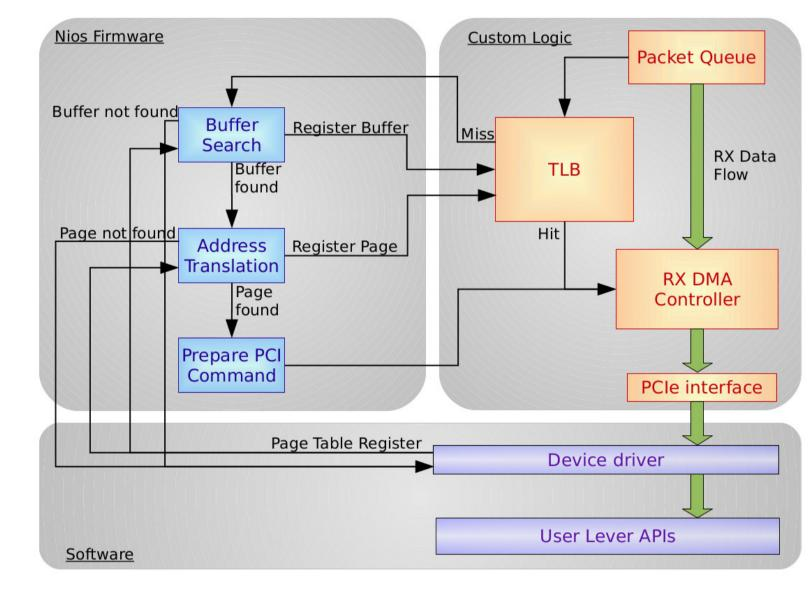
A novel implementation of a Translation Look-Aside Buffer (TLB) has been developed, to accelerate virtual-to-physical address translation at hardware level.
